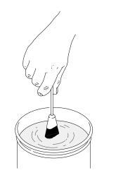
12. With the gun pointed down, clean the front of the gun, using the soft-bristle brush and solvent.
